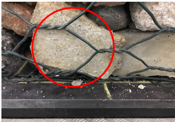
Figure 7. Failure of waste edges after the compression test performed.
