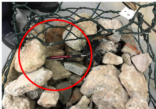
Figure 8. Inner failure of waste after compression test performed.
