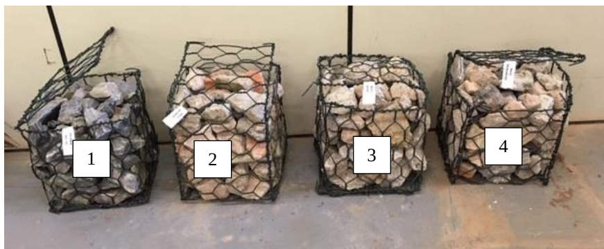
Figure 1. Test gabions filled with C&DW (2,3 and 4) and basaltic rock (1).
